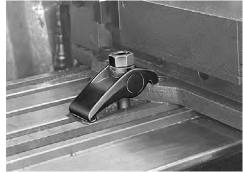
Forged Adjustable Clamp holding one side of a hydraulic vise on a milling machine table.
